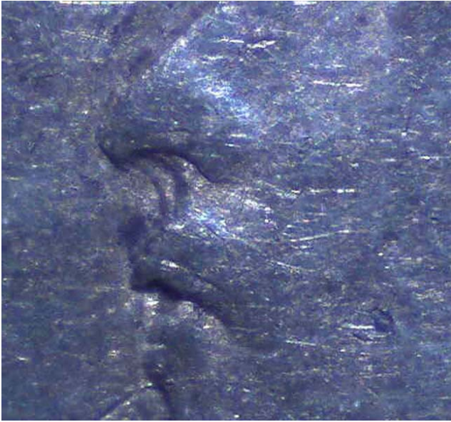
Figure 1. Doubling is very clear between the nose and upper lip. All figures magnified x60.
