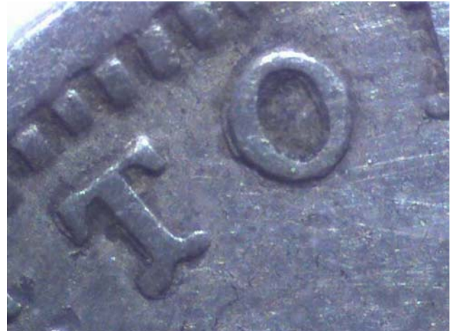
Figure 4. Note the deterioration of the base of the 'T' of VICTORIA. This effect is also especially noticeable in the 'T' of VICTORIA, the 'D' of D:G and the 'R's of VICTORIA and REG
